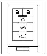
(Lock): Press to lock the doors and arm the theft-deterrent system. See *Theft-Deterrent* System on page 2-19 for additional information.
